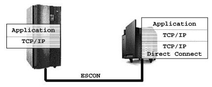
Figure 5-1. Point-to-Point TCP/IP
